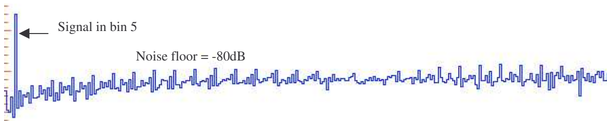
Sigma Delta ADC sine wave spectrum close up
