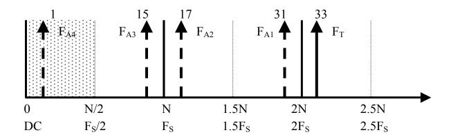
Now  $F_T$  is above two times  $F_S$  (or M is over two times N, same difference) so the waveform aliases back to the Nyquist bin, but is not reversed in time. How far can this go on? Forever. Sampling is very similar to heterodyning, and in communications now, 2.4GHz carriers are being heterodyned down to a baseband frequency of, say 40MHz, then re-heterodyned (sampled) into an ADC and decoded. There is no limit, other than what your electronic front end can handle.
