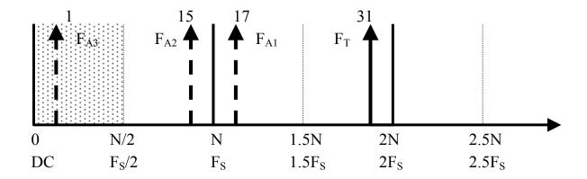
In this diagram we see  $F_T$  falling in bin M (31) but you can't see bin 31, you only get bins 0 through N/2. The image of  $F_T$  shows up in bin 17 as  $F_{A1}$ , then aliases into bin 15 as  $F_{A2}$ , and finally falls back into bin 1 as  $F_{A3}$ . Let's try applying the rules first, let's apply Rule Number One.
