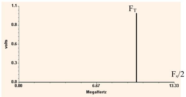
You can see here that  $F_S/2$  is going to be 13.333MHz, and if you remember that the spectrum is half the size of N then it should make sense that  $F_T$  in bin 387 is going to loom pretty high up in the spectrum, leaving no room for harmonics, at least unaliased harmonics. You should remember that what you see here is an artificial signal, so it doesn't have any harmonics, but it's not hard to create them and simulate a bad device. Just like this:
