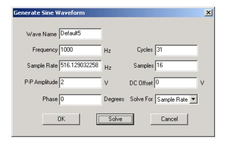
Here the sample frequency is 516Hz, and now M is 31. Looking at the time domain waveform:
