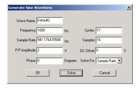
Now I've set the  $F_S$  to 941.176Hz, lower than  $F_T$  itself (still 1000Hz). This causes M to be 17, or N+1. And the waveform is...
