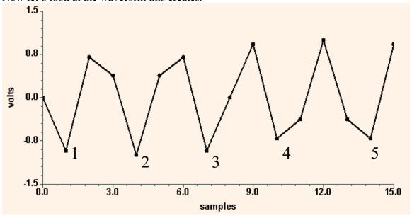
Note right away that we don't see 11 cycles, and the waveform starts by going negative despite a zero degree phase setting in our dialog box. We actually only get 5 cycles. That should be a clue to what is going to happen in frequency domain.
