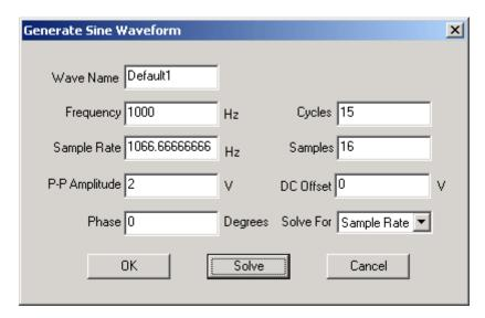
Again we use the Generate Sine Waveform dialog to create the waveform, this time  $F_S$  (Sample Rate) is 1066.66666Hz, just above  $F_T$  of 1000 Hz. We are going to be capturing 15 cycles of the waveform into 16 samples. Are you ready for the time domain representation of the waveform? I bet you're not.
