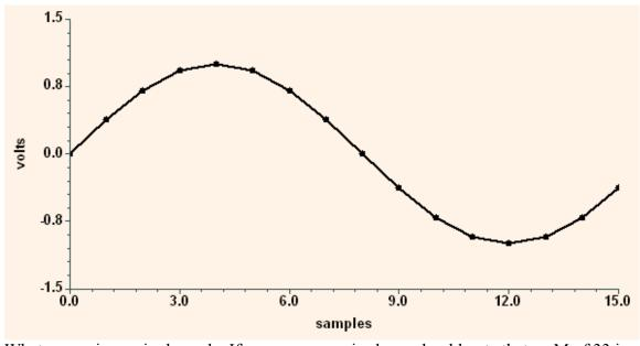
What a surprise, a single cycle. If you were surprised you should note that an M of 33 is just 2\*N+1. This waveform is equivalent time sampled. Now for frequency domain.
