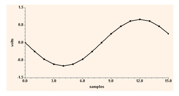
Remember we talked about equivalent time sampling, well here is another case. This happened because M is N\*2-1. In fact, if M is N times any number, minus 1, the result looks like this. Examples in this case are 31, 47, 63, 79, 95, 111, 127, etc. If M is equal to N times any number, plus 1, the captured waveform will look like one cycle, but it will be forward. Examples of this case are 33, 49, 65, 81, 97, 113, 129, etc.
