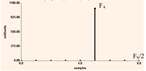
In frequency domain we see a 1V peak amplitude in bin 5, and remember, we saw 5 cycles in the captured time domain waveform, despite the fact that we had M set to 11. Let's try Dan's Aliasing Rule Number Two (does it bother you that we haven't seen rule one yet?).
