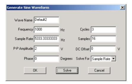
Here we are back at the Generate Sine Waveform dialog box, but this time I changed the Sample Rate  $(F_S)$  from 16KHz to 5.333333333KHz. In other words  $F_S$  was reduced by a factor of three. You'll note that I kept  $F_T$  and N the same, so the only thing that could change is M. So now when we look at the waveform generated by this dialog, it should have 3 cycles.
