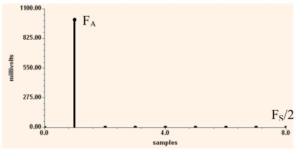
It's in bin one again. Remember that the phase is going to be reversed (because M is N\*X-1), but again, that doesn't matter. Here is what happened.
