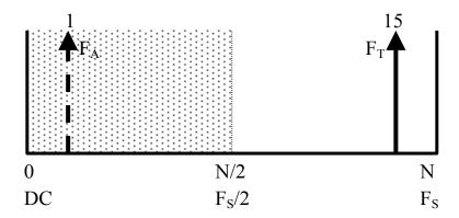
Since  $F_T$  falls into bin 15, or just one bin **below**  $F_S$ ,  $F_A$  falls into bin 1, or one bin **above** DC. That's the way aliases work, when  $F_T$  falls in the band between  $F_S/2$  and  $F_S$ , it's just like  $F_S/2$  was a mirror, with  $F_A$  being the reflection of  $F_T$ . If  $F_T$  gets closer to the mirror, so does  $F_A$  (the reflection of  $F_T$ ). If  $F_T$  gets farther from the mirror, so does  $F_A$ . Stand in front of a mirror and try it sometime.
