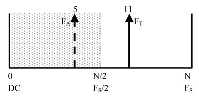
Now that  $F_T$  (which is still 1KHz) went way above  $F_S/2$  (which is now 727.27Hz) it's gone outside the Nyquist band, but it's image bounced off  $F_S/2$  and came back as an alias. Notice in this diagram how we show  $F_S/2$  equating to N/2, and  $F_S$  equal to bin N. This is true, remember that our magic sampling formula equates M to  $F_T$  and N to  $F_S$ ?
