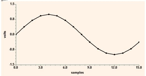
This is a single cycle of a sine wave with a frequency of 1KHz, consisting of 16 samples. The samples are separated in time by 1/16KHz (or 62.5uS), since they were captured at a rate of 16KHz. Why is there only one cycle? Because we captured 16 samples at a rate 16 times greater than  $F_T$ . How many cycles would you expect there be? If we sample every 62.5uS then 16 samples later we will have been capturing for 16\*62.5uS or 1mS, which
