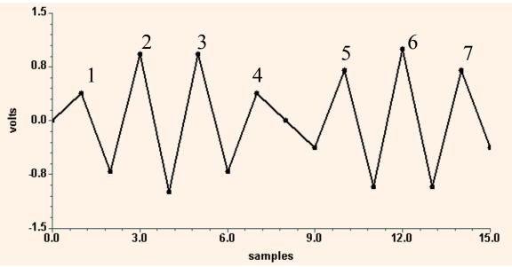
So here is the waveform, it indeed has seven cycles as noted above the waveform. Although it doesn't look much like seven cycles of a perfect sine wave, mathematically it is in fact, perfect. Just because it doesn't look so great in time domain, that's not what's important, frequency domain is what counts. Let's look.
