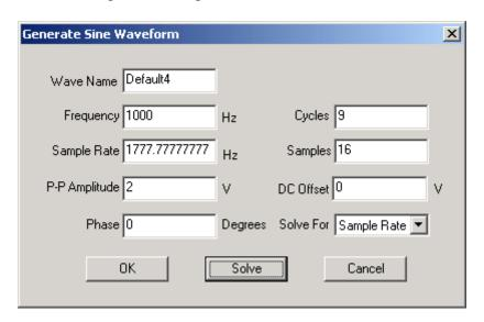
Now I've set the Sample Rate to 1777.777777Hz, which is lower than two times the test frequency  $F_T$ . Now M (the number of cycles) is 9, let's see if that really happened.
